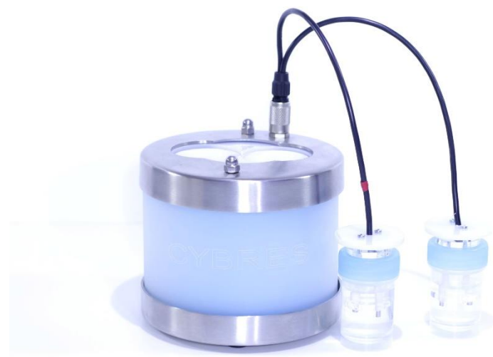
Figure 2. Differential impedance spectrometer CYBRES MU EIS, two channels with sample fluids are shown.
