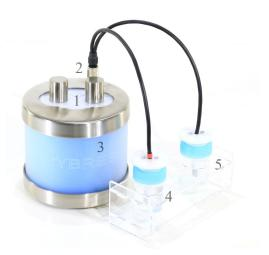
Fig. 1. The differential EIS spectrometer, 1,2,3 – elements of the device; 4, 5 – electrodes of the channel 1 and 2.
