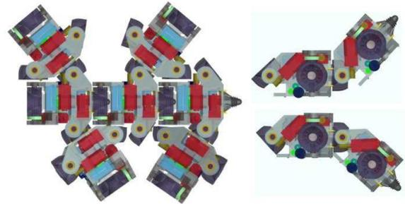
Fig. 3. Deflection of side docking connectors(±35°) and back docking connectors(±45°).
