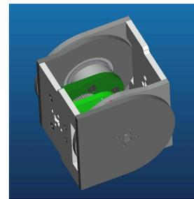
Fig. 4. Preliminary CAD design of a 1.5 DOF robot module.
