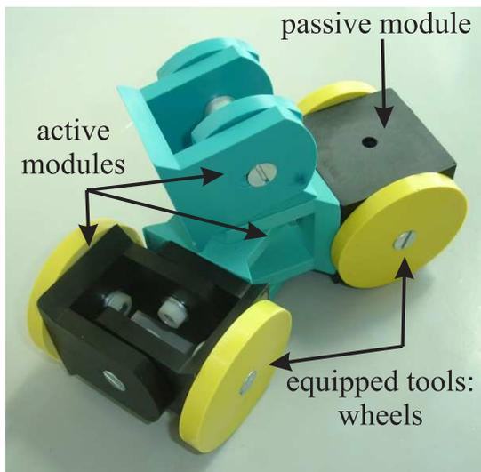
Fig. 9. "Car"-like organism, consisting of heterogeneous modules.
