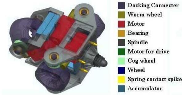
Fig. 2. CAD design a PuzzBot module with 2DOF.
