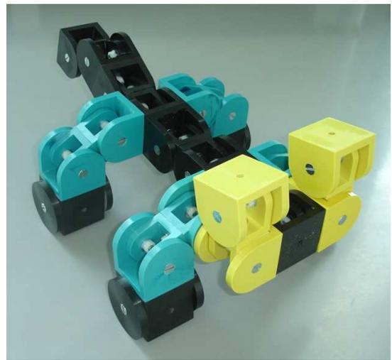
Fig. 8. "Dog"-like organism consisting of 3DOF modules with legged and wheeled locomotion.
