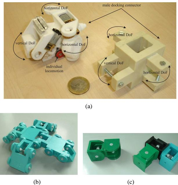
Fig. 6. Topological models of different modules. (a) (left) First rapid-prototyping model with docking elements and individual locomotion, (right) topological model of the PUZZBOT; (b) Topological models of wheeled modules; (c) Topological models of different crawling modules with 1.5 DOF and 3 DOF.
