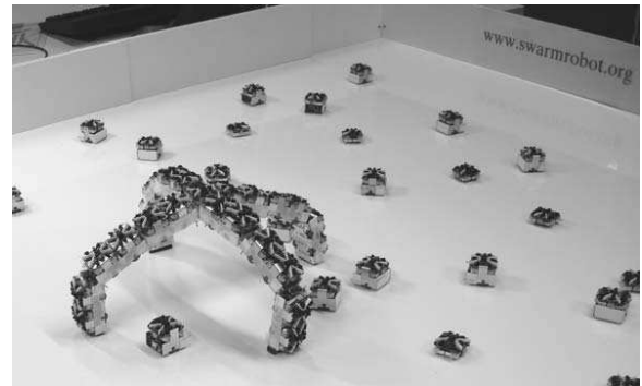
Fig. 2. Topological model of a 3D multi-robot organism. The organism possesses a common energy bus, where all robots share their energy resources.
