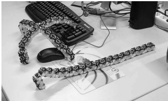
Fig. 3. Topological models of two different multi-robot organisms of different topologies and different locomotion principles.
