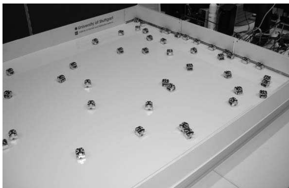
Fig. 1. Collective energy foraging in a swarm of 50 micro-robots Jasmine. Docking station consists of two copper strips with 5V installed on the back-wall. Each robot has the Li-Po recharging chip. Robots when approaching docking station are competing.
