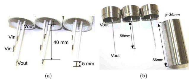
Figure 1. (a) Electrodes in the third setup; (b) Electrodes in the fourth setup. Images are from (Kernbach, 2013b).
