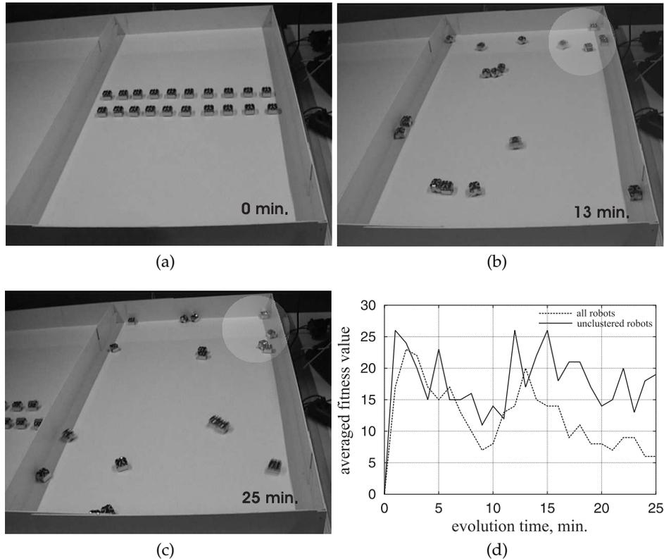
**Fig. 2.** Course of the experiment: (a) Start; (b) 13 minutes; (c) Finish; (d); The light spot in (b) and (c) shows clustered robots. Changes of the averaged fitness value during 25 min. of experiments.
