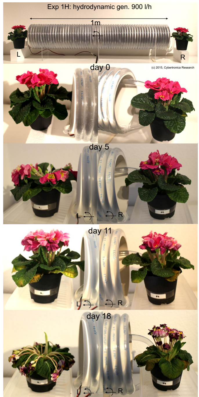
Fig. 23. The experiment 1H with the hydrodynamic generator and biosensors – flowers primula acaulis , the pumped water volume is about 900 l/h. Watering was carried out every 1.5-2 days (otherwise plants dry out) by the 'wet-floor' approach equally for L and R flowers.
