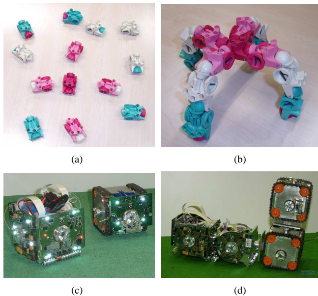
Figure 1. (a) Prove-of-concept: individual robots; (b) Prove-of-concept: aggregated robots into an artificial organism; (c) Real prototypes: individual robots; (d) Real prototypes: aggregated robots (images ©SYMBRION, REPLICATOR projects).
